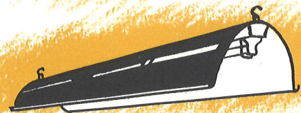
High mounting — trough type — used for H3000-A9 mercury lamps.
